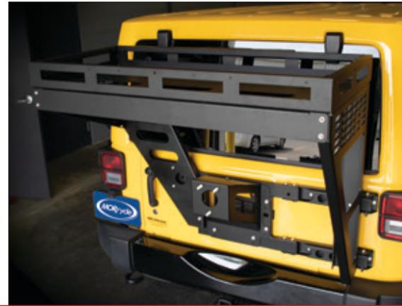
Perfectly designed to carry gear on overland and off-road expeditions. Mounts to the MORryde heavy-duty tailgate reinforcement and heavy-duty tailgate hinges.
