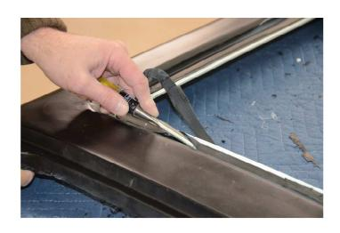
4. Finished. It took a little less than 30 minutes work to get to this point, both windows of a JK Unlimited hardtop could be removed in about an hour. A 2-door might take slightly longer because the windows are longer - there's more adhesive to cut.
