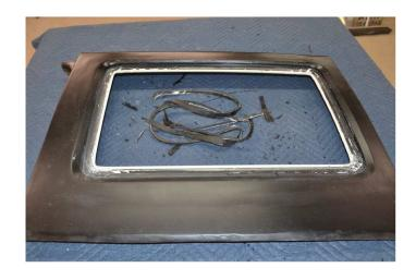
The window opening will need to be trimmed slightly in order to fit the slider window. Cutting can be done with an angle grinder with a cutting disk, a jigsaw with a very fine tooth blade or abrasive cutting blade installed (don't use a large-toothed blade as it may crack the fiberglass), or an air die grinder with a coarse sanding disk. Final adjustment can be done with sandpaper or a file.
