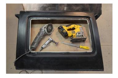
5. Set the retrofit kit frame in the window opening. Any of the original window opening that lies inside the opening in the retrofit kit must be trimmed away using one of the tools described above. A Sharpie marker can be used to trace the inside of the opening on the hardtop.
