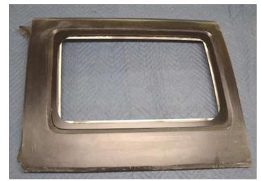
6. Once the holes is cut, set the retrofit kit back in place and note any areas which will need adjustment – using sandpaper or a file remove any additional material necessary so that the window opening in the hardtop matches the inside opening of the retrofit kit. The result should looks something like this.
