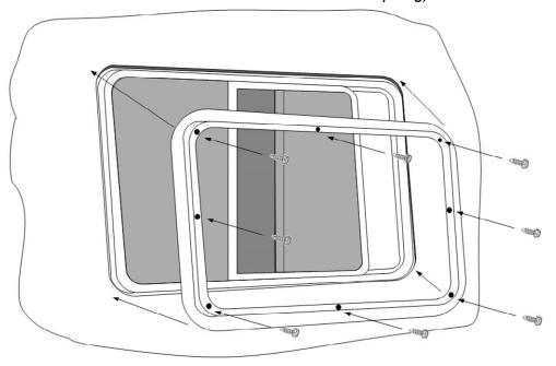
When installing the window/retrofit kit assembly, ensure that compression weatherstrip you applied in step 9 is in contact with the caulk you applied in step 10 all the way around the frame.
