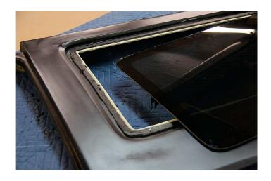
3. A sharp chisel or scraper makes quick work of removing the remaining adhesive.
