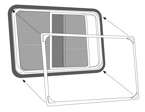
9. Apply the bulb weatherstrip to the inside of the retrofit kit frame. The weatherstrip should be even with the outside edge of the retrofit kit frame. The weatherstrip should ends should meet at the bottom of the frame, and should be trimmed for a tight joint.
