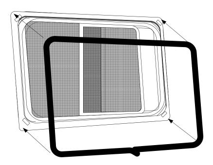
10. Apply a bead of caulk to the inside of the window recess in the hardtop. The caulk should be along the corner where the window mounting surface joins the sides of the recess.
