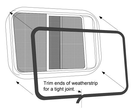
8. Remove the protective paper from the weatherstrip you applied in step 1 and install the retrofit kit frame to that weatherstrip. Push the retrofit kit frame and the window frame together all the way around to ensure a good bond between the window frame, weatherstrip, and retrofit kit frame.
