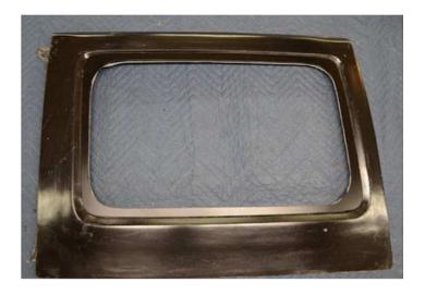
Once the opening is trimmed, the window and retrofit kit can be installed.
