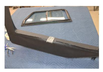
Tip 3: To remove a stubborn bulge, double-sided tape can be used on the inside of the weatherstrip. The canvas can be pulled tight and stuck down to the tape before the clamp ring is screwed into place.
