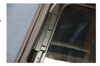
Step 7: Screw bracket into window frame. The screws will go through the bracket and through the holes in the clamp ring and will self-drill into the v-groove on the outside of the window frame. A nut driver (shown) is the best tool for this because there's no risk of a screwdriver slipping out of the slot and damaging the window.
