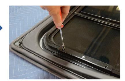
Step 8: Drill holes in the frame of the upper for the screws which will secure the bracket to the upper. Since the screw heads of the screws installed in the previous step may interfere with drilling, they can be removed one at a time while each hole is drilled and reinstalled before moving on to drill the next hole.
