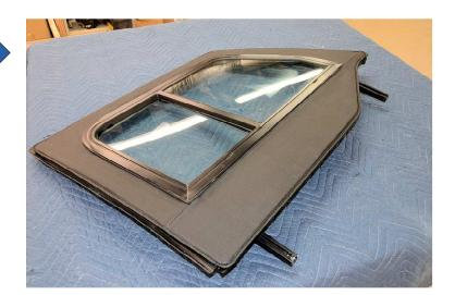
Tip 1: Bulges in the canvas can happen if the hole in the hole in the canvas is a tight fit around the window. In most cases the fit can be improved by trimming a little more off the bottom of the hole
