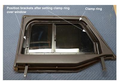
Brackets should be positioned so the holes in the bracket line up with holes in the clamp ring. The outside edge of the bracket should be touching or close to the inside of the plastic upper frame. (If you're installing the windows in Bestop or Rugged Ridge uppers, your brackets will be different – see page 6 for instructions for installing those brackets.)
