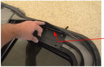
Undo Velcro and slip bracket under metal rod frame. Secure bracket to frame with zip ties through holes in bracket. Ensure the zip tie clasp is on the inside of the door, pull tight, and trim excess\*.
