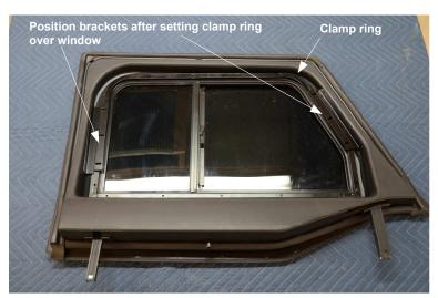
Step 5: Temporarily drive a few screws through the clamp ring holes into the window frame. Once the screws are in, turn the assembly over and check the fit. If the canvas is bulged anywhere, the following steps will help achieve a flat fit.
