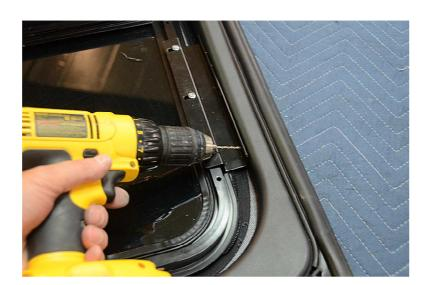
Step 8: Drive screws into the holes drilled in the previous step. Because of the position of the screws, a 1/4" open end or box end wrench will be easier to use for this step than the nut driver.
