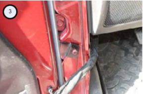
Left: The top bolt of the lower door hinge is removed and reinstalled to secure the bottom tab.
