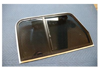
Step 4: Insert the slider window into the opening from the outside. Flip over and place the clamp ring over the inside of the window, and position the brackets so the holes in the brackets line up with the holes in the clamp ring. Ensure the window is centered so that the brackets will be able to screw into the clamp ring and into the plastic frame of the upper.
