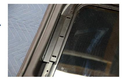
Step 5: Screw bracket into window frame. The screws will go through the bracket and through the holes in the clamp ring and will self-drill into the v-groove on the outside of the window frame. A nut driver (shown) is the best tool for this because there's no risk of a screwdriver slipping out of the slot and damaging the window.
