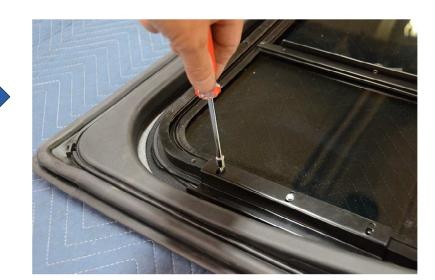
Step 6: Drill holes in the frame of the upper for the screws which will secure the bracket to the upper. Since the screw heads of the screws installed in the previous step may interfere with drilling, they can be removed one at a time while each hole is drilled and reinstalled before moving on to drill the next hole.
