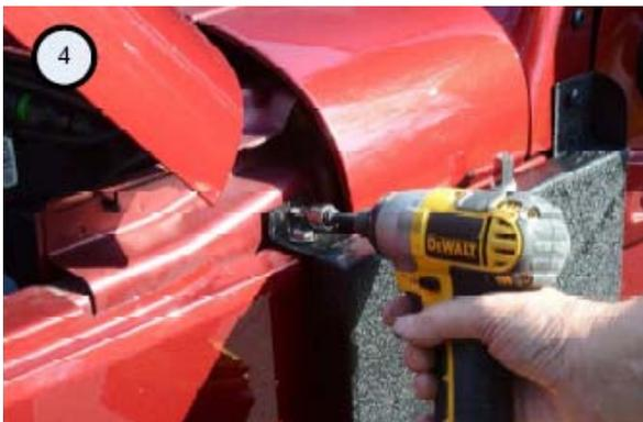
Removal Instructions: The Side Mount is designed so that it can be easily and quickly removed when carrying extra fuel isn't necessary - just remove the 3 screws/bolts (or 4 if you've installed the optional self-drilling screw). The hinge bolt and the Torx screw should be reinstalled when the Side Mount is removed, and it's a good idea to reinstall the 5/16" bolt and the self-drilling screw so they don't get lost for the next time you install the Side Mount.
