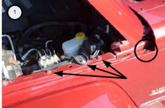
Left: There is an existing hole in the fender into which a j-nut needs to be inserted (circled). It may be necessary to temporarily remove the fender bolts indicated by the arrows, so the fender can be flexed outward slightly to allow clearance for the j-nut to be installed.
