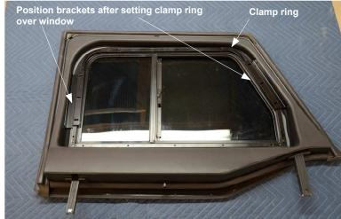
Brackets should be positioned so the holes in the bracket line up with holes in the clamp ring. The outside edge of the bracket should be touching or close to the inside of the plastic upper frame.
